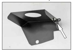
8. Install the heat shield mounting bracket (064313) onto the heat shield as shown using the provided hardware.
