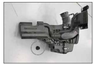
9. Remove one of the mounting grommets from the factory air box.
