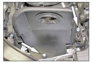
14. Install the heat shield assembly so that the mounting grommet is on the air box mounting stud and the bracket aligns with the bolt hole from the previous step, secure the heat shield using the factory bolt from the previous step.
