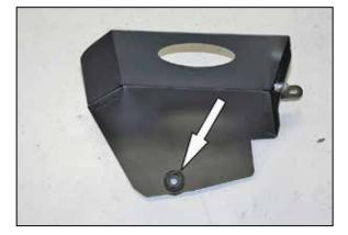
10. Install the mounting grommet into the heat shield as shown.
