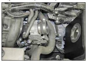
15. Install the provided coupling hose (084036) onto the throttle body and secure with the provided hose clamp.
